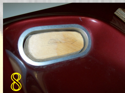
8 The wood should pass easily through the opening with at least a 1/8" gap all the way around. The space is needed for the screen to fit. Sand the wood for a perfect fit.
