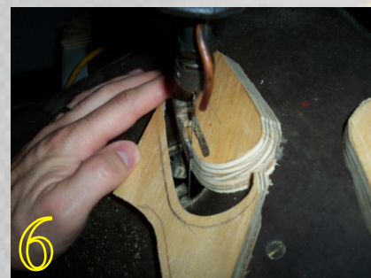
6 Cut the wood on the inner line with a band saw or jig saw, with the blade set at a 45 degree angle.
