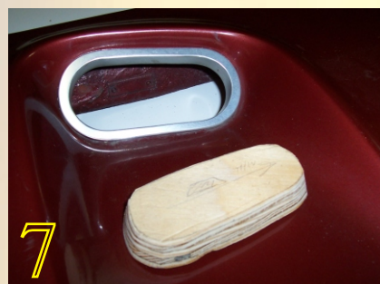
7 After you cut the wood parts, match them to the vents LH and RH because some Sterling openings are right and left handed.
