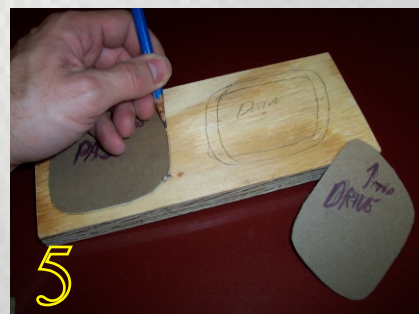
5 Trace the templates onto a 1/2" thick piece of wood. Then, offset to the inside the line you just traced another line 3/8" from the first line.
