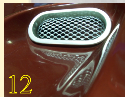
12 This is the completed, formed screen vent on my Sterling. Note that some owners glued door edge molding neatly into the vent, and others painted the edge to set them off. The billet aluminum rings on mine are "L" shaped so the small end slides into the hole. A local machine shop can make these for you if you trace the opening, or I can provide engineering drawings.
