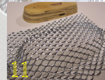
11 The completed screen, ready to trim to fit behind the vent opening.
