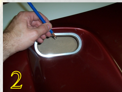
2 First step is to trace all your vents onto a stiff cardboard or posterboard. Make sure to mark them LH or RH, top/bottom and inside/outside
