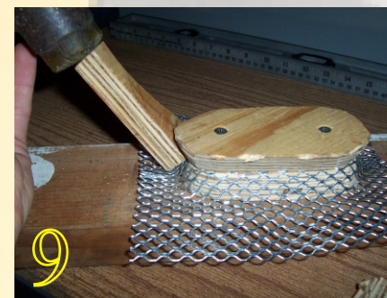
9 Start to hammer the mesh down around the parts you made. Hammer onto a rounded block of wood, and work your way around the form until the screen sits close. If the screen breaks, insert another piece and try again! Notice the LH and RH blocks are face to face, so I could hammer either direction.
