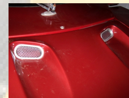
New mesh intakes. I used adhesive to glue them in place from underneath. Notice how they curve out and look refined and more complex.
