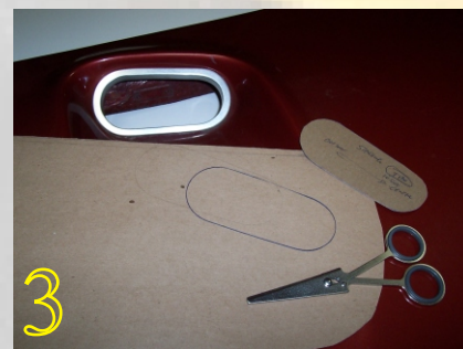
3 Next, cut the templates and fit them inside the openings. Trim as needed so there is a 1/8" gap all the way around.
