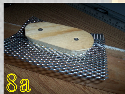
8a Now the fun begins! Screw the LH and RH wood parts together with the new vent screen between them. Use long screws so both parts can be secured directly to each other and into a solid surface for stability. Gutter Gard screen is a common screen, but any can be used as long as it's flexible.
