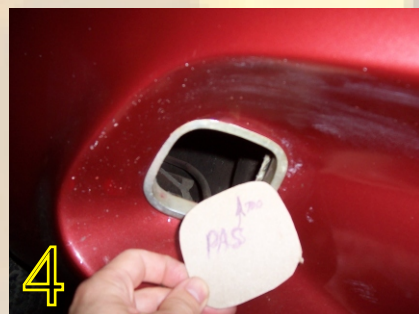
4 Make certain you make templates for all four vents on your Sterling. They may all be a little different in size. The lower side vents are different from each other, too.
